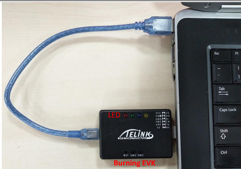
Figure 2-2 Connect “ Burning EVK ” with PC
